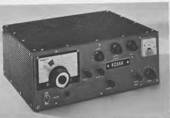
Front view of WA2ELL's and K2SKK's mobile 50-watt transmitter. Unit measures approximately 12 inches in width, 5 inches in height, and 10 inches in depth.
